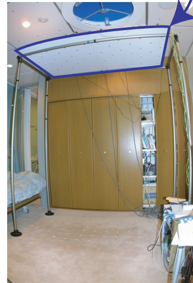
Figure 7: Experimental system for locating a human head by ultrasonic radar
