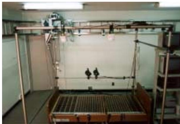
Fig. 1 Pressure distribution monitoring sheet set on bed
