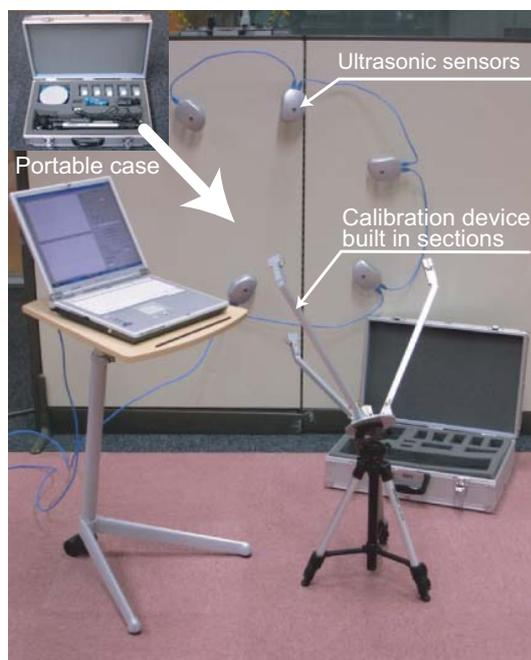
Fig. 12. Developed portable ultrasonic 3D tag system
