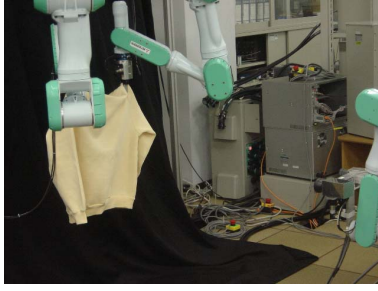
Figure 1: System consisting two manipulators and stereo cameras
