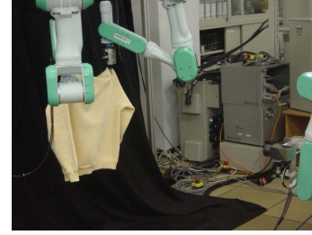
Figure 6. System consisting of two manipulators and stereo cameras
