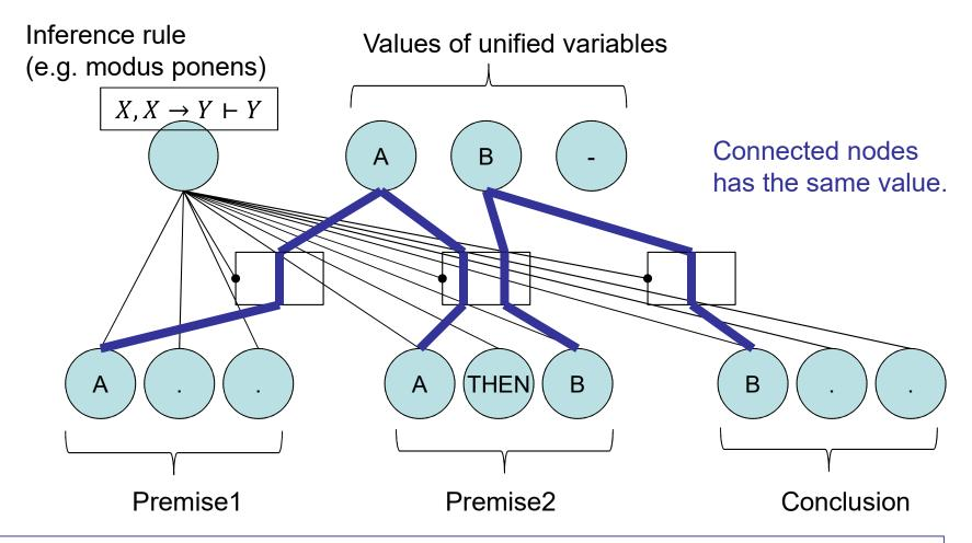
The network can infer not only a conclusion from the premises, but also the premises from a conclusion. The network will be able to learn inference rules from sample data of premises and conclusions. This mechanism will become key technique to implement unification grammar parser such as CCG.
