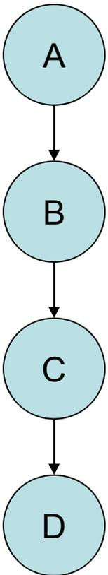
$$\begin{aligned} P(A, B, C, D) \\ = P(D | C)P(C | B)P(B | A)P(A) \end{aligned}$$
