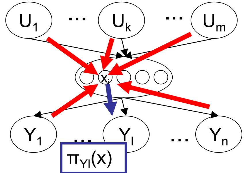
$$\lambda_X(u_k) = \beta_2 \sum_x \lambda(x) \sum_{u_1, \dots, u_m / u_k} P(x | u_1, \dots, u_m) \prod_{i \neq k} \pi_X(u_i)$$
