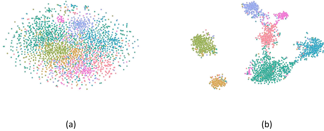
Fig. 8. Figure shows t-SNE embedding plots of the node features of Cora dataset. Each node belongs to one of the seven classes represented by different colors. (a) Plot of initial node features, (b) Plot of node embeddings learned after training FSGNN model on the dataset.
