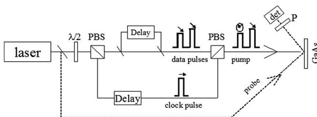
FIG. 3. Experimental setup for the study of the recording speed for spin-photon memory.
