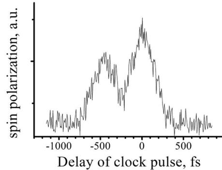
FIG. 4. Spin polarization of electrons excited by combined beam of clock pulse and two data pulses as a function of delay of clock pulse. For each point, the delay length was  $(n+1/4)\lambda$ , where  $n$  is an integer. Reading of spin polarization was done 100 ps after arrival of pump pulses.
