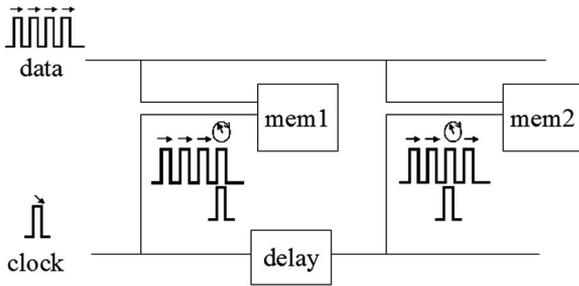
FIG. 2. The scheme for the integration of memory cells. Pulse diagrams explain the method for the high-speed recording.
