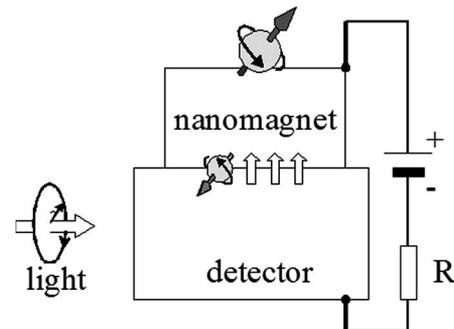
FIG. 1. Design of spin-photon memory cell. A bit of data is stored as magnetized direction of nanomagnet. For the data recording, the circularly polarized light creates spin-polarized electrons in the detector. Injection of these electrons into the nanomagnet causes magnetic torque, which turns the magnetization of nanomagnet, and the data is memorized.
