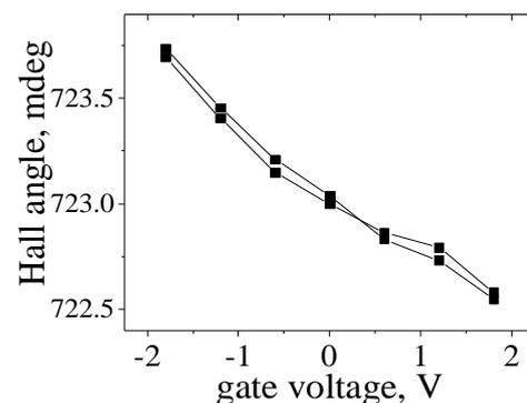
Figure 3. Hall angle as function of the gate voltage in FeB film
