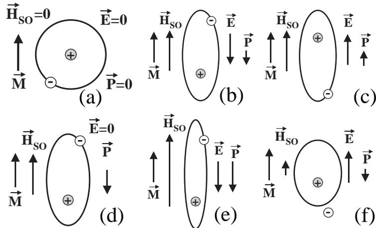
Fig.6. Deformation of electron orbital under a gate voltage. Ellipses show lines of constant electron density in the close proximity of the nuclear. (a),(d)  $V_g=0$ ; (b),(e)  $V_g>0$ ; (c),(f)  $V_g<0$ . Without gate voltage, the orbit is (a)-(c) centrosymmetric; (d)-(f) elongated toward the gate. The gate location is under orbital.  $\mathbf{P}$  is the net electrical polarization,  $\mathbf{M}$  is the magnetization and  $\mathbf{H}_{SO}$  is the effective magnetic field of SO interaction.
