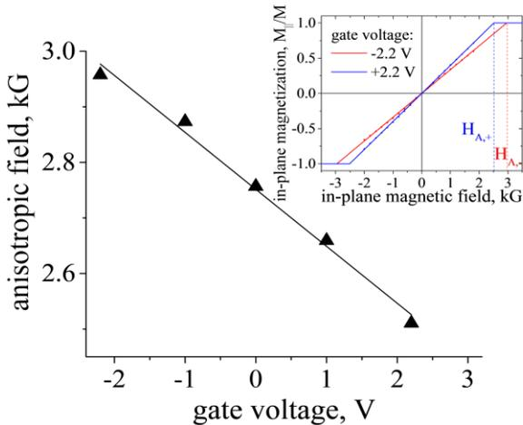
Figure 4. Anisotropic field vs gate voltage in FeB film. Inset shows in-plane magnetization as a function of the in-plane magnetic field.  $H_{A,+}$ ,  $H_{A,-}$  are anisotropic fields for  $V_{gate} = +2.2$  V,  $-2.2$  V respectively.
