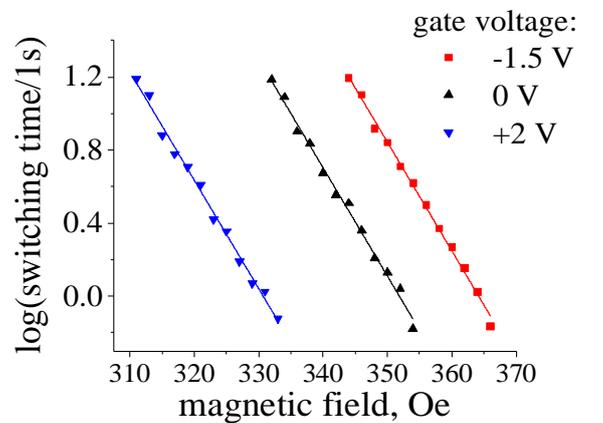
Figure 5. Magnetization switching time in FeB/W multilayer as a function of the perpendicular magnetic field. The line crossing with the x-axis ( $y=0$ ) gives the coercive field of 363, 351, 330 Oe and the crossing with y-axis ( $x=0$ ) gives retention time of  $10^{21.66}$ ,  $10^{20.88}$ ,  $10^{19.64}$  seconds at  $V_{gate} = -1.5, 0, +2$  V, respectively.
