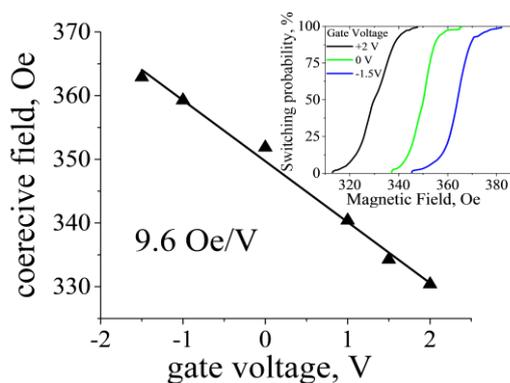
Figure 2 Coercive field vs voltage measured in FeB/W multilayer. Inset shows switching probability from magnetization-up to magnetization-down direction as function of the magnetic field
