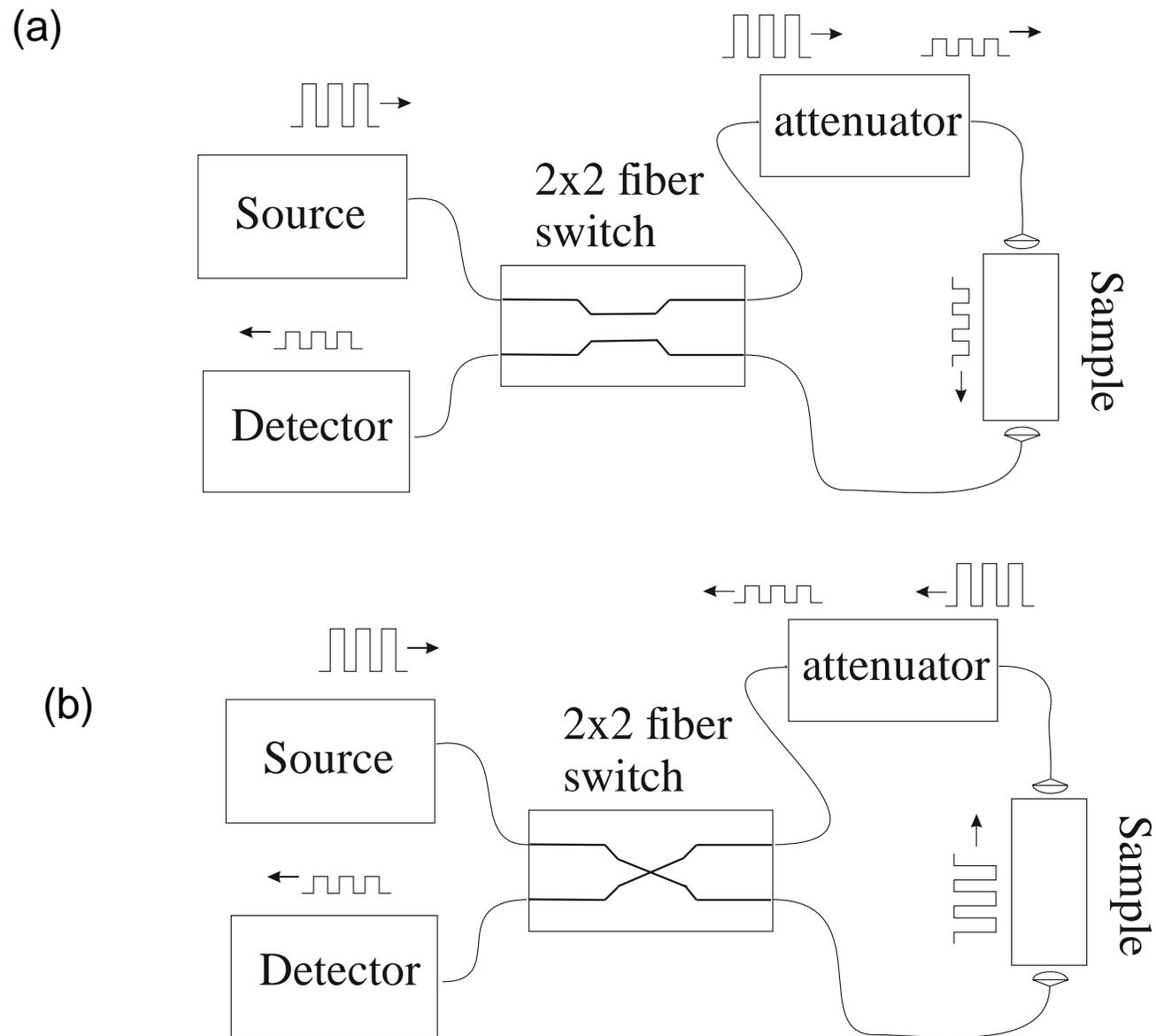
Fig.10 the setup for measurements of non-linear absorption. (a) and (b) show two switch states of the switcher. For different switching states, light of different intensity passes through the sample, but light of nearly- same intensity reaches the detector. A train of pulses shows the intensity of light at different points
