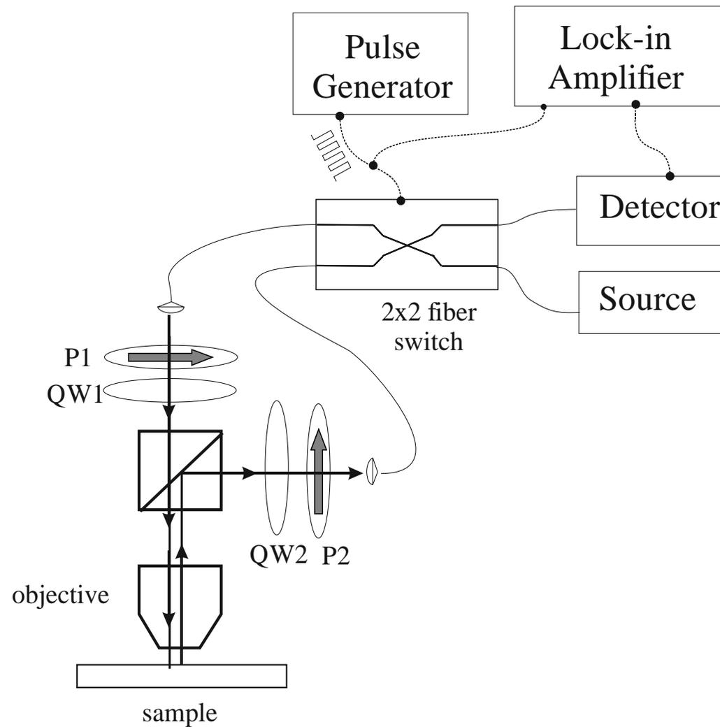
Fig.11 the setup for measurements of Kerr rotation angle. The angle between axes the polarizers P1, P2 is 45 degrees. The angle between axes quarter-wave plates QW1,QW2 and the polarizers are + 45 and -45 degrees.
