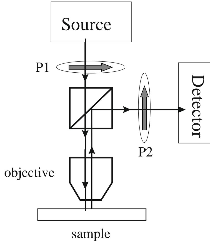
Fig.4 Prior Art. Conventional setup for measurements of Kerr rotation angle. Polarized light from the source is reflected from the sample and it is detected by the detector. The angle between axes of polarizer (P1) and analyzer (P2) is 90 degrees and light is blocked. Only when the polarization is rotated after the reflection, light reaches the detector and the rotation angle can be evaluated.
