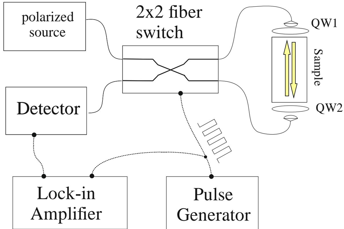
Fig.9 the setup for measurements of the MCD. A polarized light source, polarization-maintaining fibers and fiber switch are used. The quarter-wave plates QW1 and QW2 are inserted between collimators and sample.
