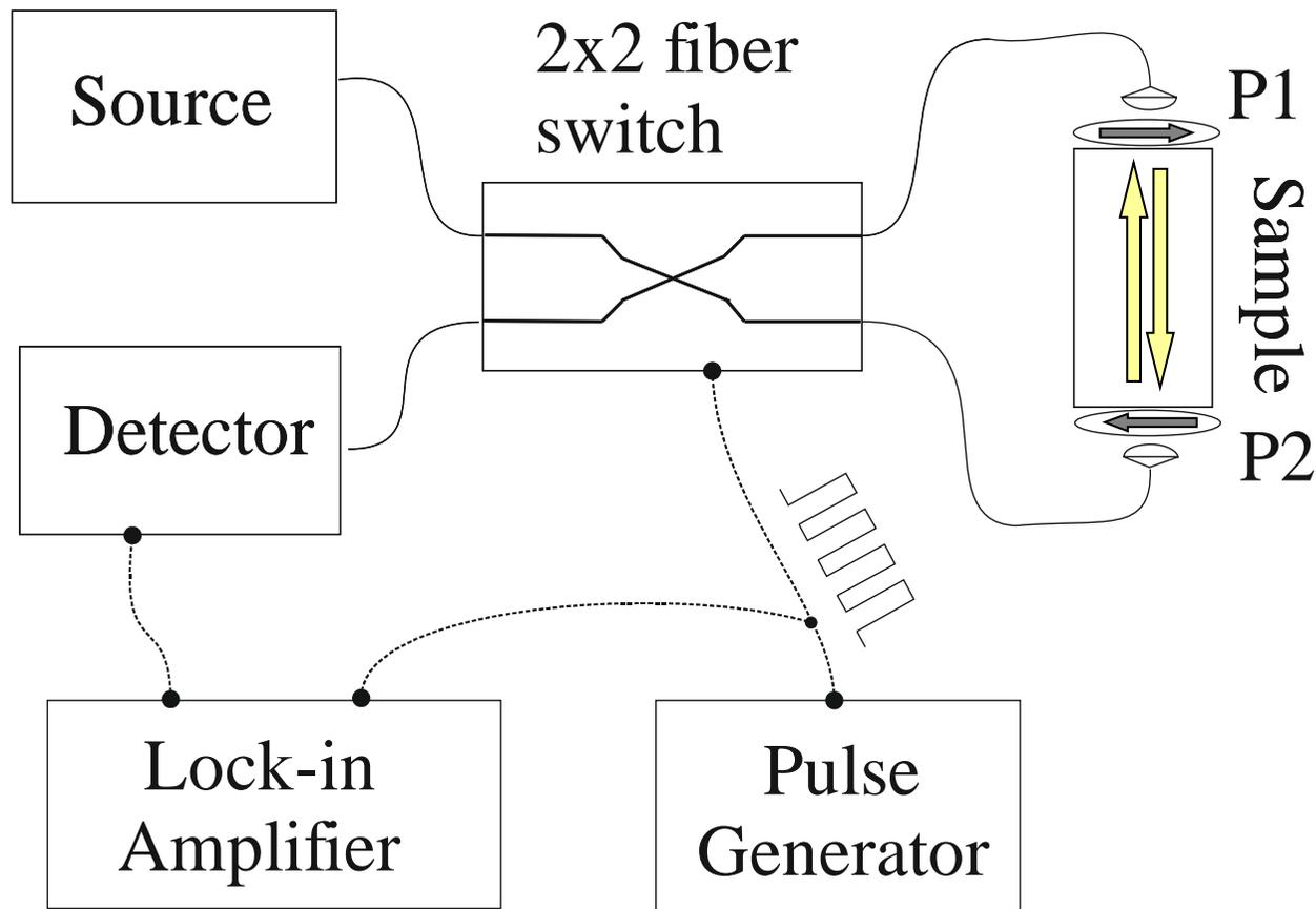
Fig.7 the setup for measurements of the Faraday rotation. The polarizers P1 and P2 are inserted between the fiber collimators and sample. The angle between axes of the polarizers is 45 degrees.
