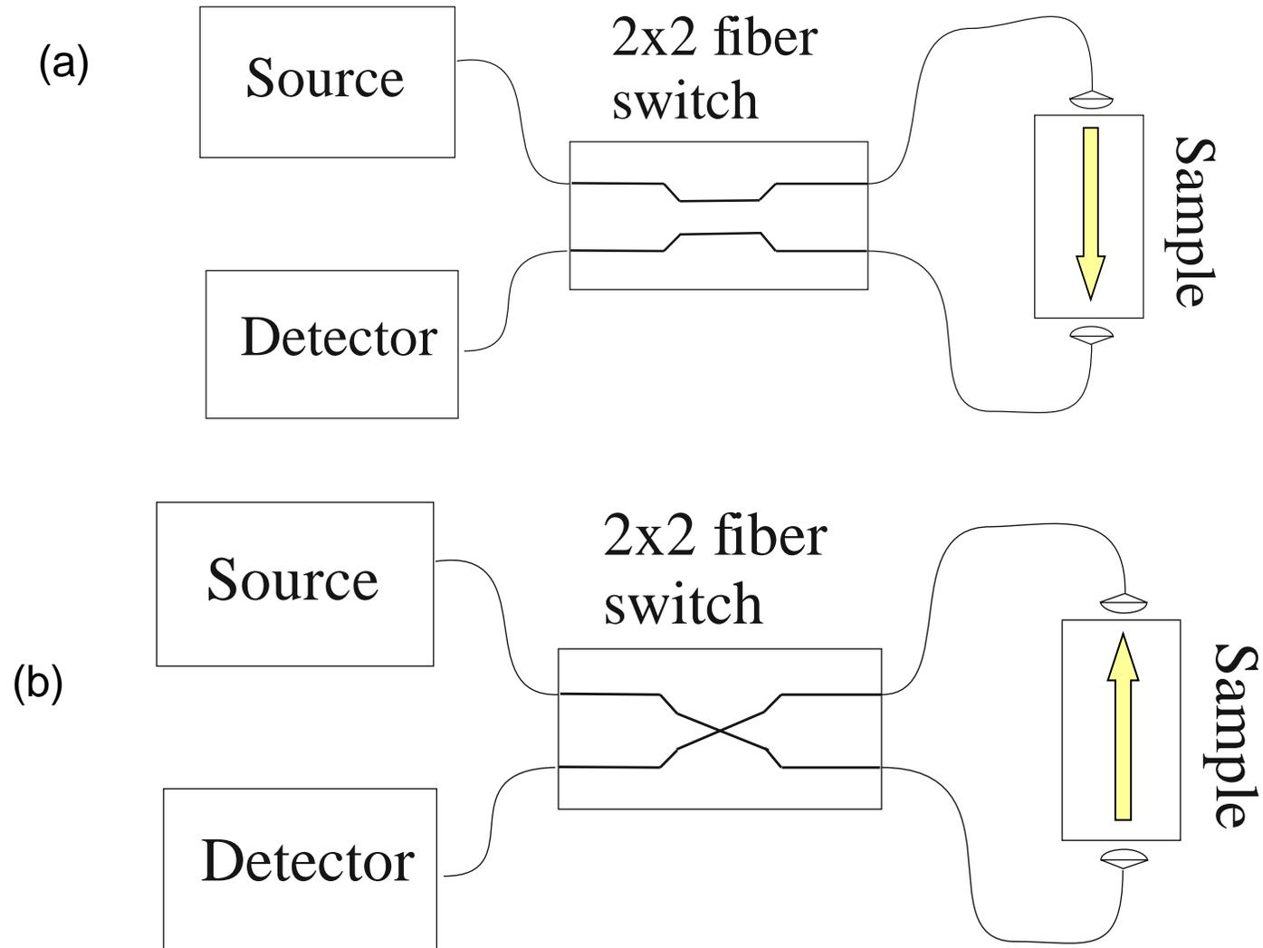
Fig.5 the setup for measurements of the non-reciprocal loss. Fig. 5 (a) and (b) show two switch states of the switcher. The yellow arrows indicate the directions of light propagation.
