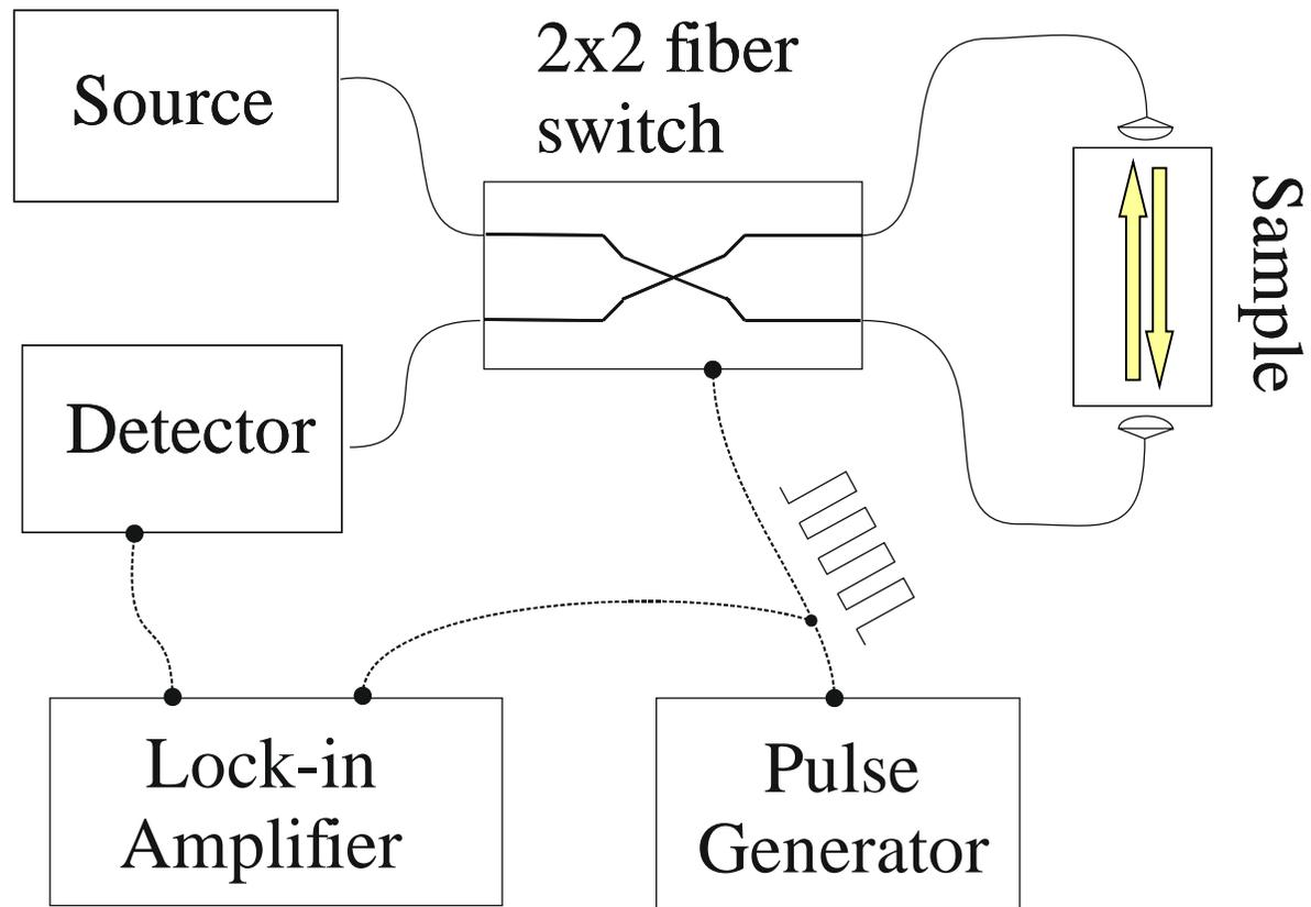
Fig.6 the setup for measurements of the non-reciprocal loss using lock-in technique
