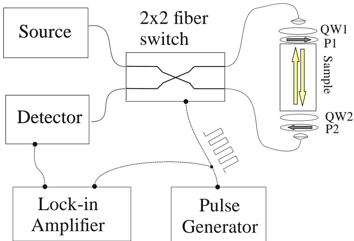
Fig.8 the setup for measurements of the MCD. The quarter-wave plates QW1 and QW2 are inserted between polarizers P1 and P2 and sample. The axes of the polarizers are in the same direction. The angle between axes of polarizers and QW1 is 45 and between polarizers and QW2 is -45 degrees
