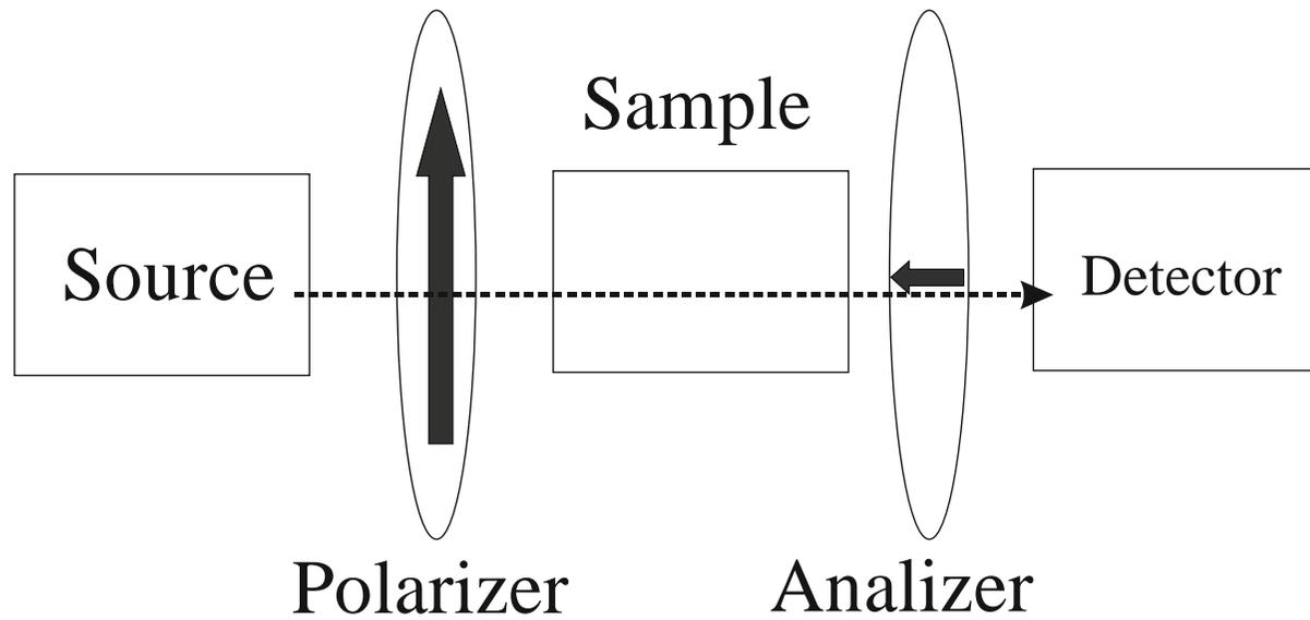
Fig.1 Prior Art. Conventional setup for measurements of Faraday rotation. The sample is placed between crossed polarizer and analyzer, which block the light propagation from the source to detector. When the polarization is rotated by the sample, light can reach the detector and the rotation angle can be evaluated.
