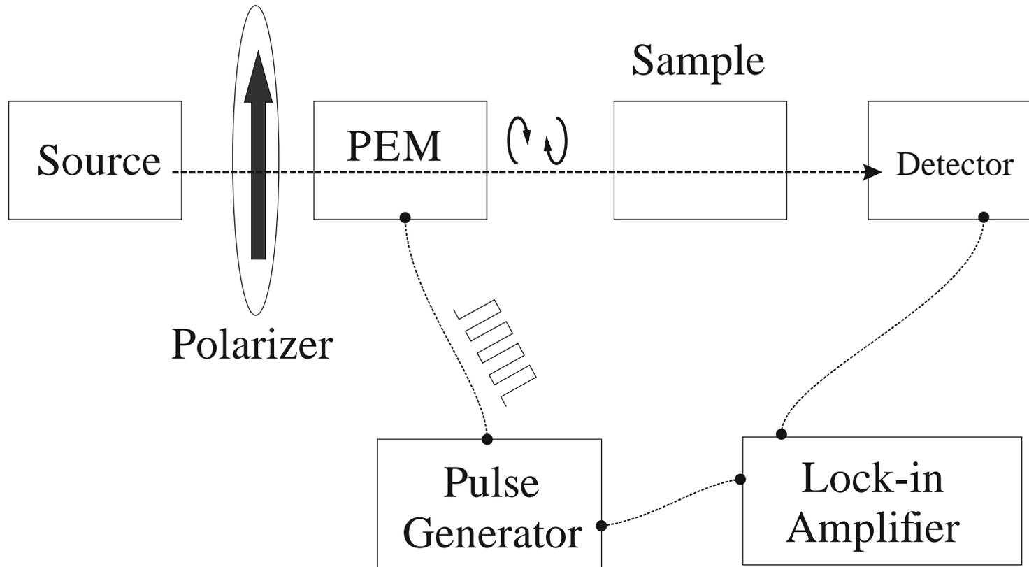
Fig.3 Prior Art. Conventional setup for measurements of magnetic circular dichroism (MCD). After the photo-elastic modulator (PEM) the polarization of light becomes modulated between left- and right- circular polarizations. The difference in absorption between left- and right- circularly polarized light is detected by the detector using the lock-in technique.
