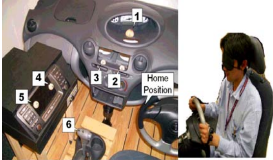
Figure 5: Experimental Driver's Cockpit. Left: Targets and Home Position of Driver's Hand. Right: Subject Driver wearing an eye mask and the 3D-position tracker on the left hand.
