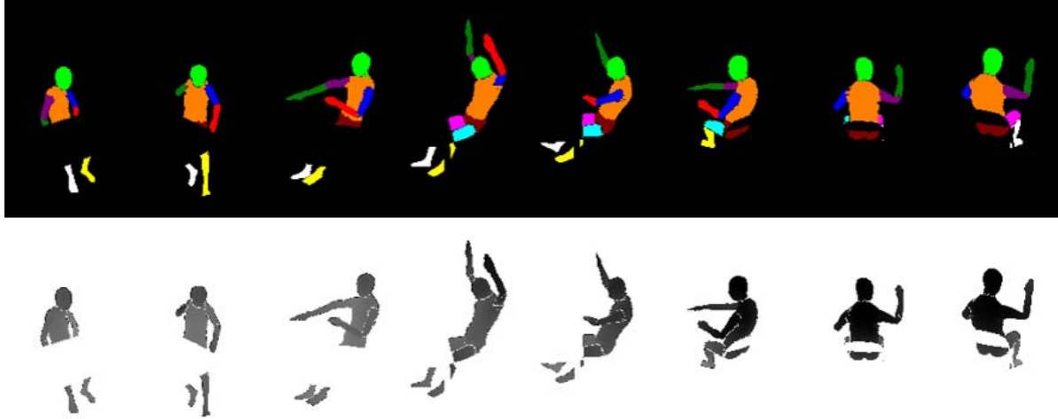
Figure 11: Example pairs of body part label images (first row) and depth images (second row).
