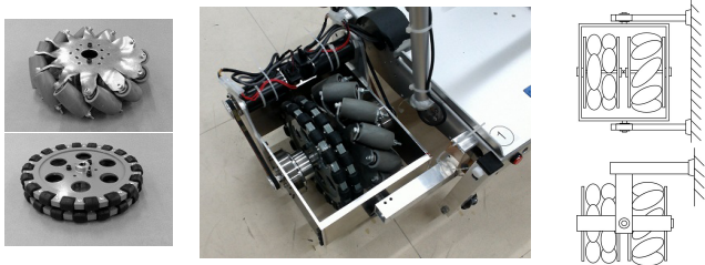
Fig.2 A mecanum wheel and omni-wheel (left), the zoomed photo of a mecanum omni-wheel unit (center) and its top and front view figure of the gimbal suspension (right)
