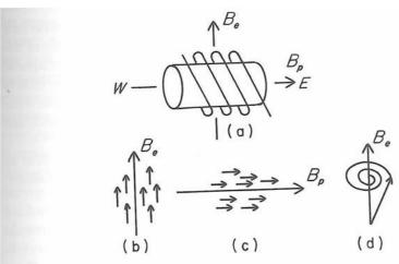
Fig. 7.11. Principle of the proton magnetometer.
