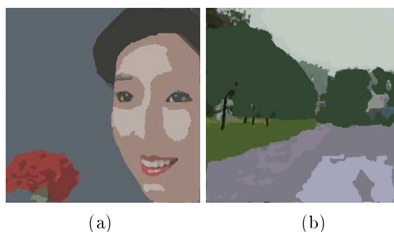
Figure 6: Segmentation result by combining the restricted region growing. (a) Face. (b) Outdoor.
