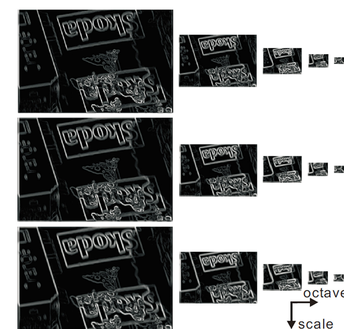
Examples of multiresolutional edge images. Multiresolutional orientation maps are obtained by computing the orientation maps for each edge image.
