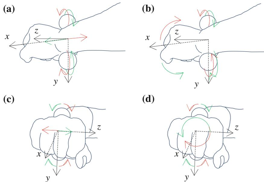
**Fig. 2** Concept sketch of guidance in four axes ( $x$ ,  $yaw$ ,  $z$ , and  $roll$ ). **a** Guiding in  $x$  axis. **b** Guiding in  $yaw$  rotation. **c** Guiding in  $z$  axis. **d** Guiding in  $roll$  rotation
