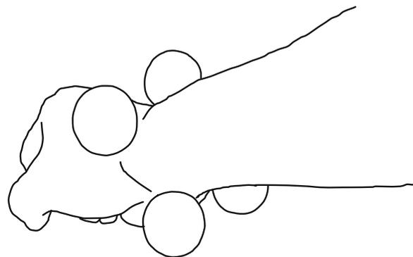
algorithm for hand motion control. Additionally, in order to provide guidance with six axes of motion, we will develop wOCHD that has four ball effectors where additional two balls are for *y* axis and *pitch* rotation (Fig. 4).
