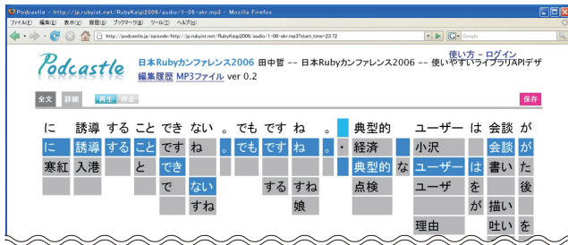
Figure 1: The error correction interface in PodCastle (competitive candidates are presented underneath the normal recognition results). Five errors in this excerpt were corrected by selecting from the candidates.
