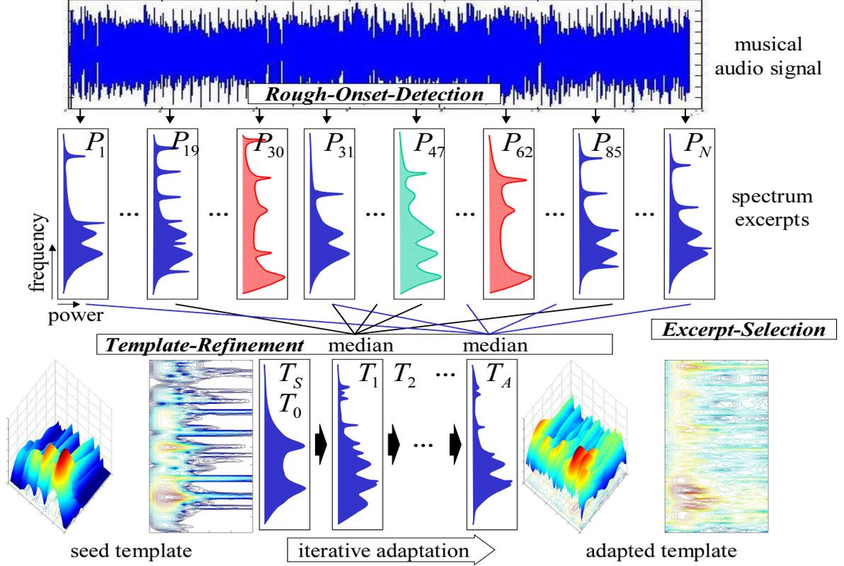
Figure 1: Overview of template-adaptation method (iterative adaptation algorithm).
