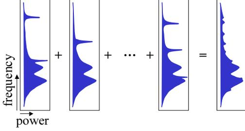
Figure 4: Updating the template by calculating the median of selected spectrum excerpts.
