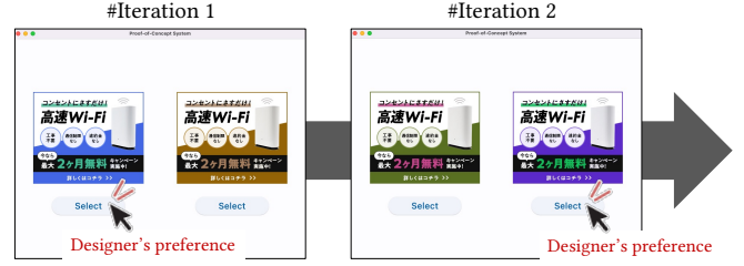
Figure 5: User interface of our banner ad design system in color editing mode. This system provides pairs of design candidates for each iteration.
