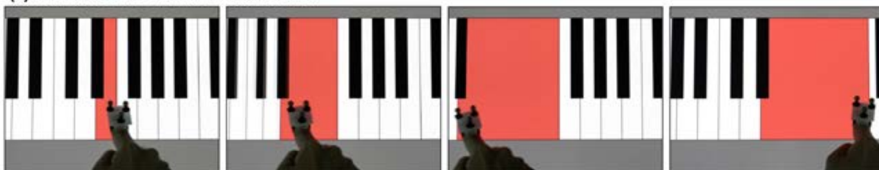
Figure 5. Implementation and use of pitch bend. The time goes from left to right while the finger moves around the correct key position. The sound from MIDI varies from four semitones below to four semitones above. When too sensitive, users can change the rate of magnification. The pitch changes in accordance with the vertical position of the finger and reflects the distance from the indication key.
