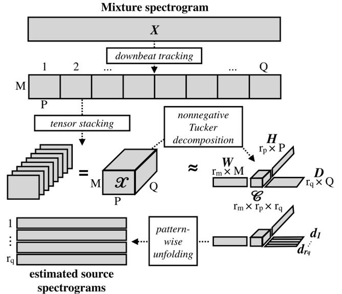
**Fig. 1.** Algorithm pipeline: the mixture magnitude spectrogram  $X$  is divided into measure-length fragments; these are stacked into a tensor  $\mathcal{X}$ ; the tensor is factorized; the pattern activations in  $D$  are unfolded one at a time into  $r_q$  estimated source spectrograms.
