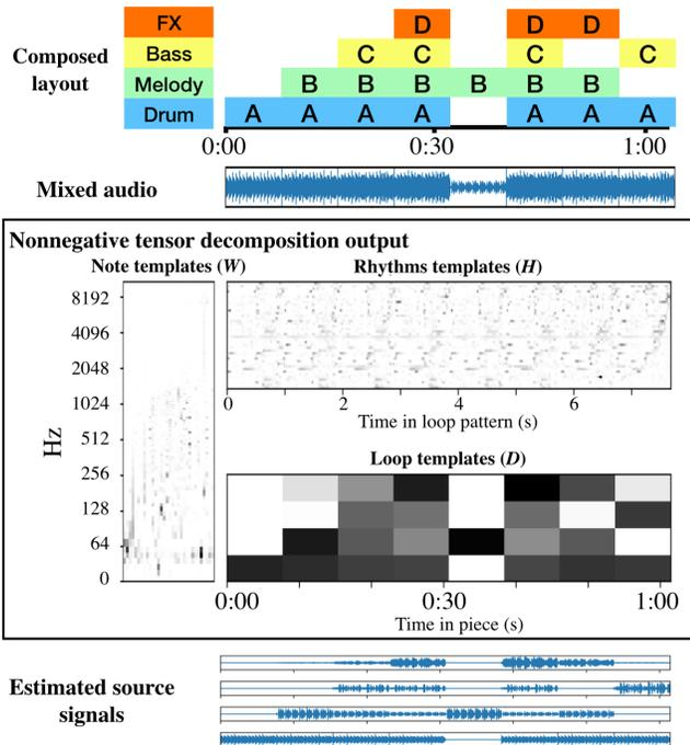
**Fig. 2.** Example input and output of the system. Top: *composed* layout of a loop-based piece of music. Middle: estimated templates corresponding to the notes, rhythms, and loop types in the audio. Bottom: source-separated signals.
