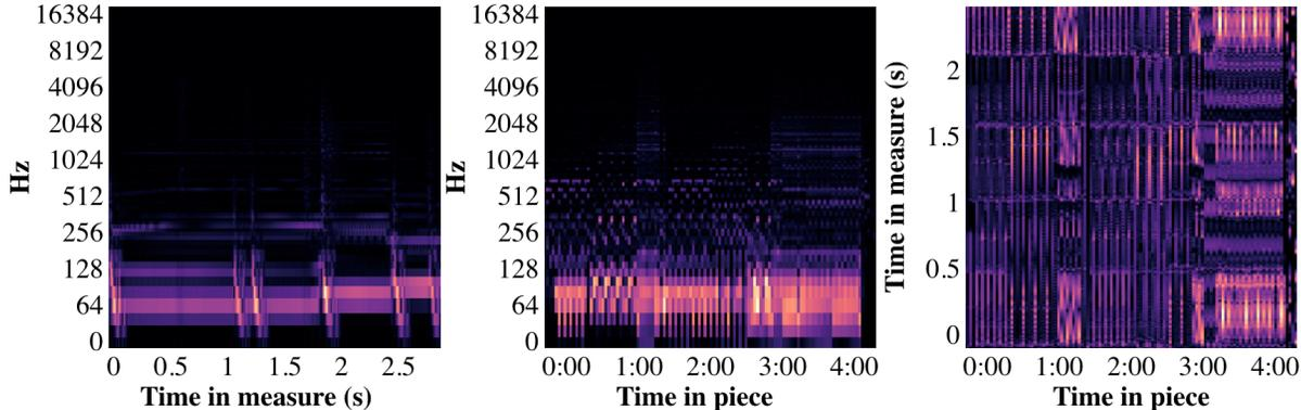
**Fig. 3.** Three slices of the spectral cube  $\mathcal{X}$  constructed for the song “El Pico” by Rataat. From left to right: (a) a single measure; (b) a single metrical position (the second beat onset); (c) a single frequency bin (pointing to the E above middle C).
