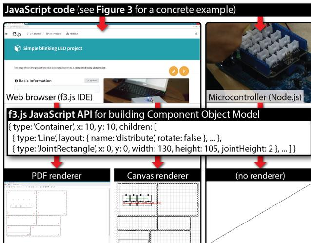
**Figure 8.** Single codebase runs on Web browsers for rendering and on microcontrollers for physical computing.
