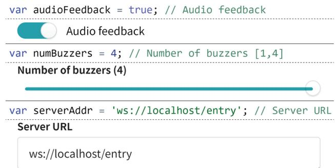
Figure 5. Variable declarations with special comments and corresponding GUI widgets.
