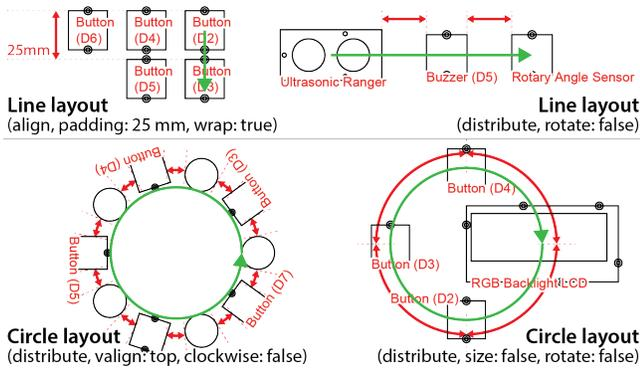
**Figure 6.** Example usage of PUI layout managers.
