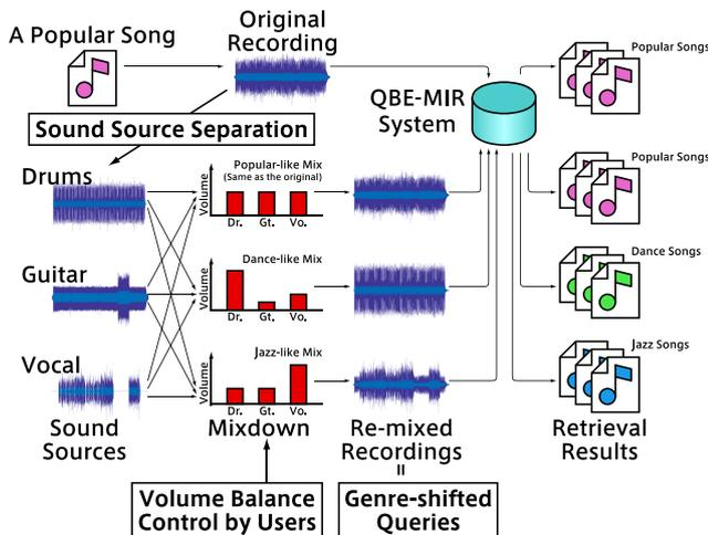
Figure 1: Overview of our QBE retrieval system based on genre shift. Controlling the volume balance causes the genre shift of a query song and our system returns songs that are similar to the genre-shifted query.
