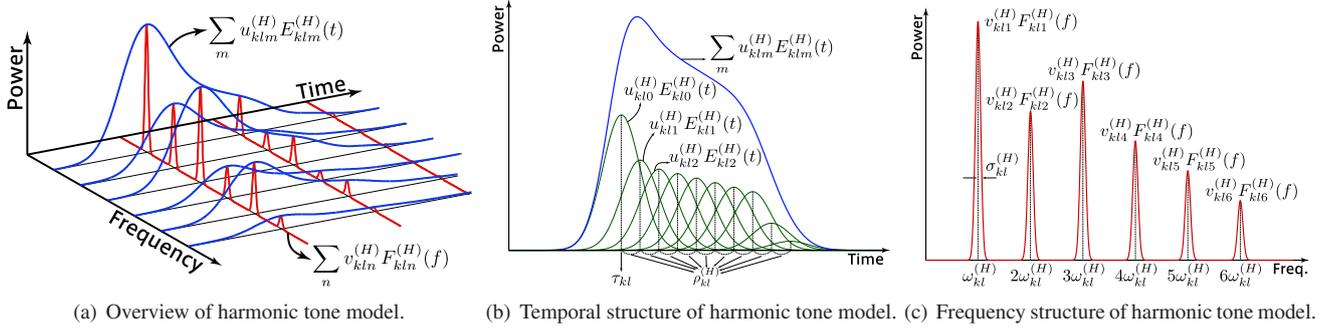
Figure 2: Overall, temporal and frequency structures of harmonic tone model. Harmonic tone model consists of a two-dimensional Gaussian Mixture Model, and is factorized into a pair of one-dimensional GMMs.
