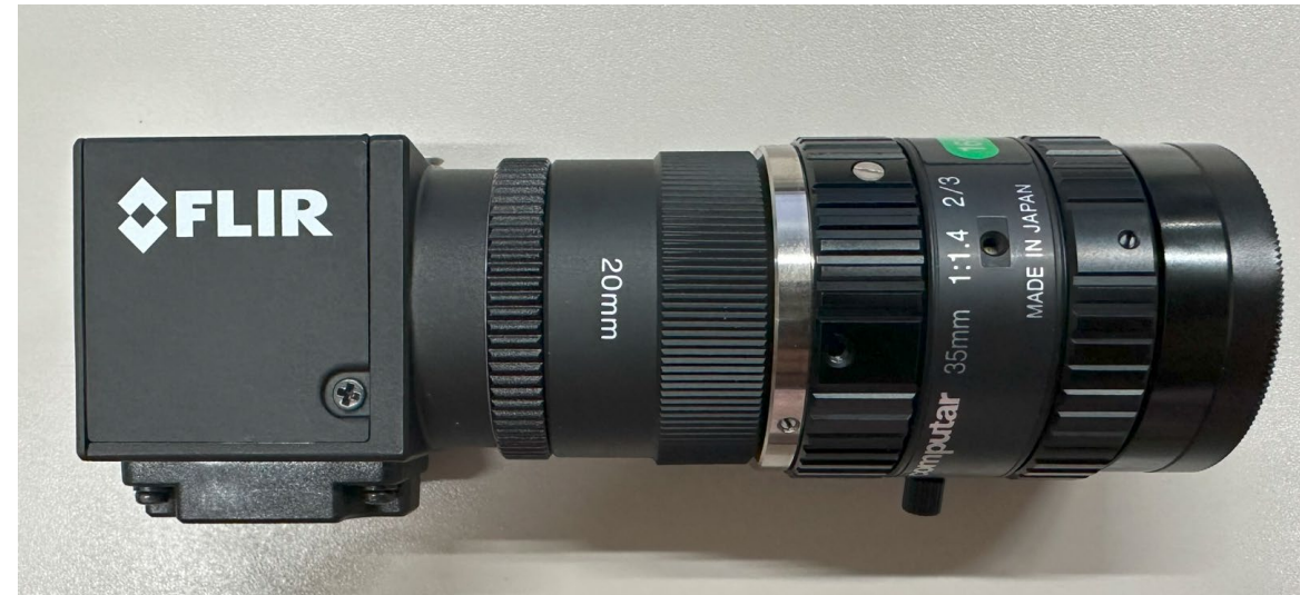
The photo shows the BFS-U3-04S2M-CS with the C/CS mount adapter.
