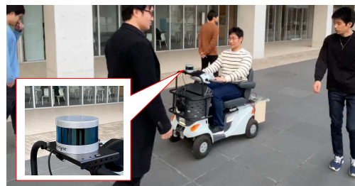
Fig. 1. Example of a personal mobility vehicle in walking space. The wheelchair is equipped with a relatively small LIDAR.
