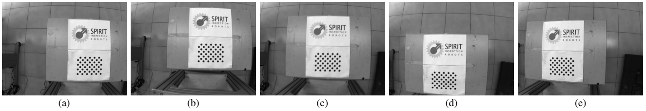
Fig. 5: The image sequence recorded while the robot was drawing a sine curve above the calibration pattern.
