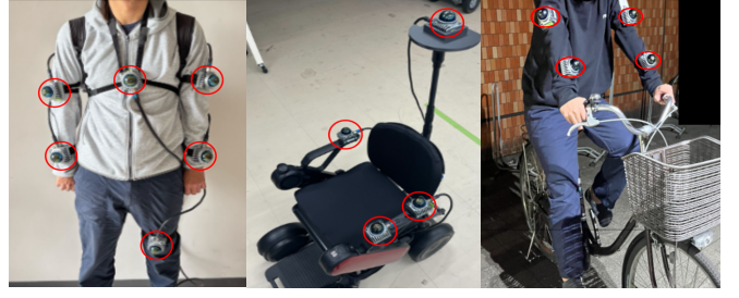
Fig. 5. Data collection. We use multiple sensors, which enables the efficient collection of data representing diverse motion patterns.
