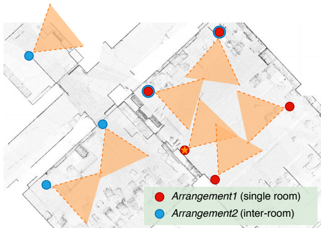
Fig. 6: The evaluation environment. Five Kinects are placed in a single room in Arrangement1 , while they are placed in multiple rooms in Arrangement2 such that they are completely separated. The Kinect marked with a star is removed later to reduce the camera overlap.
