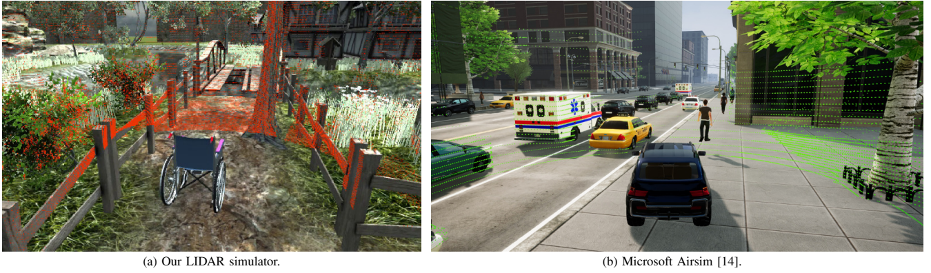
Fig. 2: Examples of point clouds generated by our simulator and Microsoft AirSim. AirSim generates point clouds from collision models, and thus objects in the LIDAR data have shapes that are too simplified (see the points on the trees, cars, and buildings), and objects without collision models (pedestrians) do not appear in the point clouds. Our simulator performs raycasting on an omnidirectional depth image to generate realistic point clouds.
