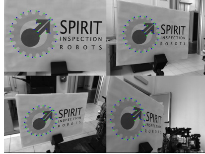
Fig. 10: The images for reconstruction and the keypoint correspondences.
