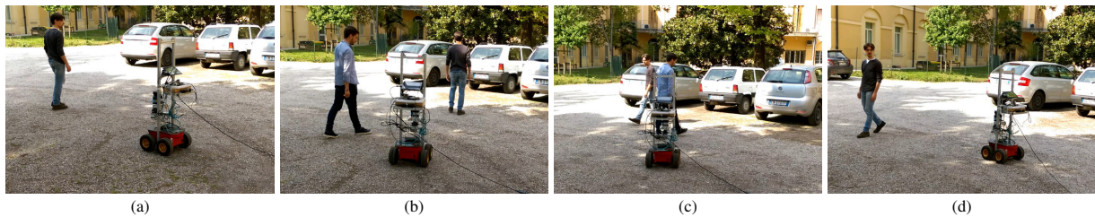
Figure 16: The outdoor person following experiment. The robot successfully kept tracking and following the target person even the target was occluded by the other one several times.
