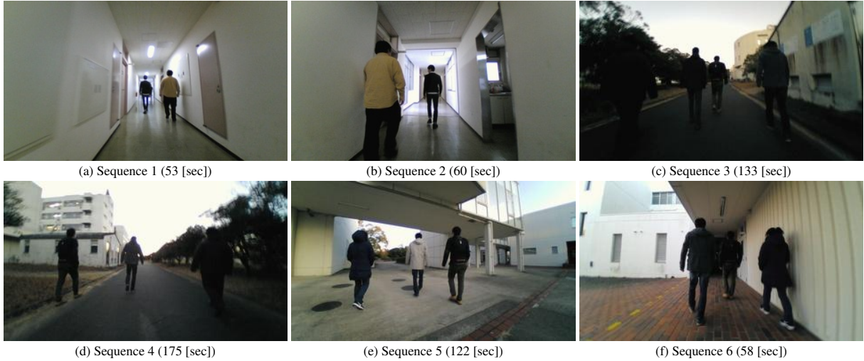
Figure 9: Snapshots of the dataset for person identification evaluation in person following tasks. The dataset consists of RGB images and LRF data recorded from a mobile robot. The robot was manually controlled and following a person in indoor and outdoor environments.
