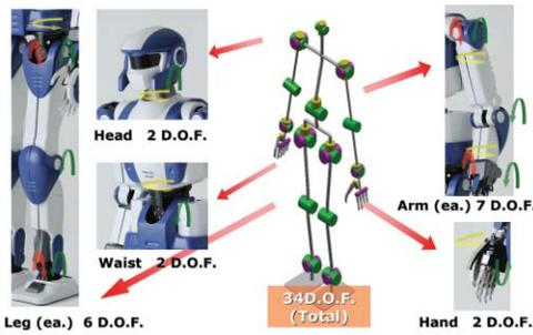
Fig. 3. D.O.F. Configuration of HRP-4
