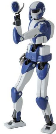
Fig. 1. Humanoid robotics platform – 4 : HRP-4
