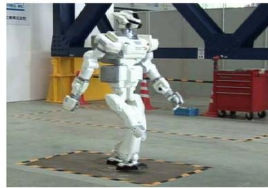
Figure 12. Demonstration of walking on a low friction floor
