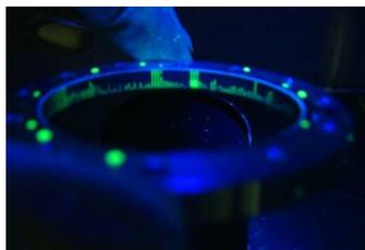
Figure 6. Splash-proof test results using a gear box of HRP-2
