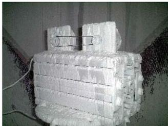
(b) Gear unit after dust-proof test
