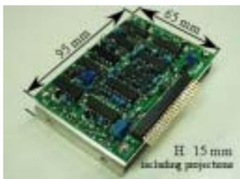
**Figure 7:** DC Motor Driver Module for 2-Axes
