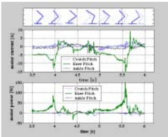
Figure 8: Current and Torque at Forward Walk
