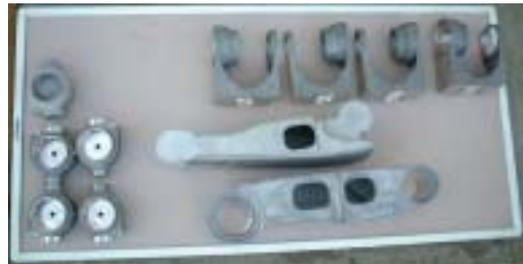
Figure 8. Magnesium Cast Links
