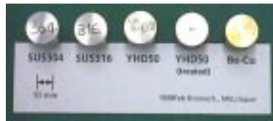
Fig. 1. Sample chips. From left, stainless steel type 304, type 316, YHD50, surface treated YHD50, and Be-Cu.
