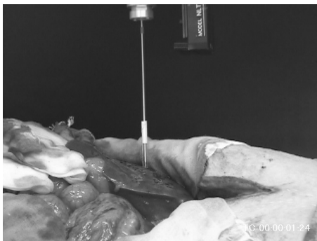
Fig. 6. Experimental set-up of constant speed insertion.
