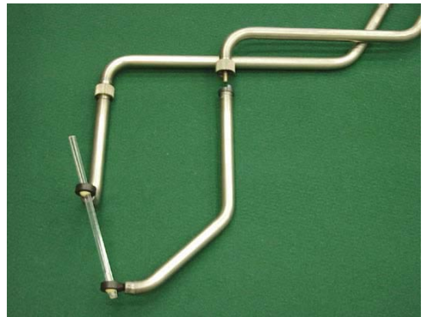
Figure 5: The rigid arms and the pivotal joints. The arms can be divided into parts small enough to be autoclaved.
