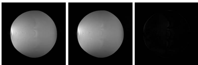
Figure 6: Images of the spherical phantom when the robot was not installed (left) and when one axis of the robot was in motion (center). The subtraction of these images showed no shift (right).
