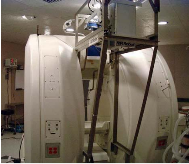
Figure 3: The constructed robot installed with the intraoperative MRI.
