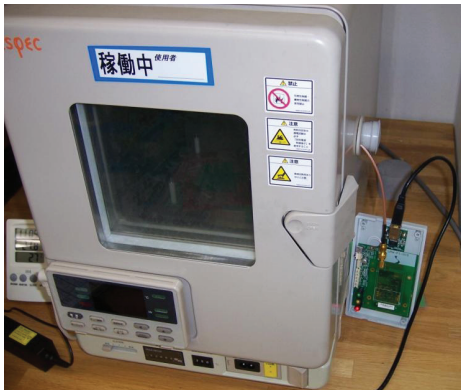
Fig. 7. PUF-embedded RFID used in the experiment.
