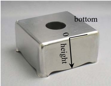
Fig. 17. Example of rectangular box shapes formed using rotational pass set. The angle of growth was 4 deg and the forming height was 30 mm.
