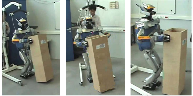
Fig. 1. An experiment of whole-body pivoting manipulation.
