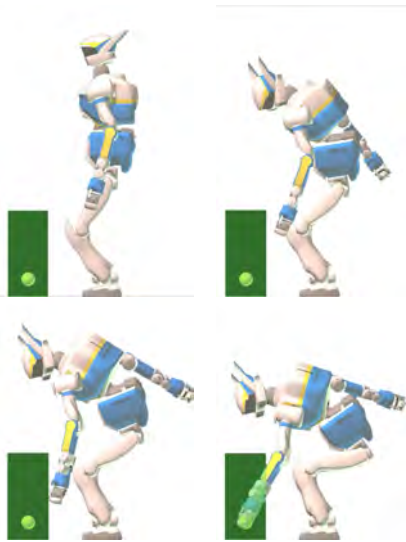
Fig. 6 Hierarchical inverse kinematics, including inequality constraints. Humanoid HRP-2 has the high-priority task of reaching the ball on the ground under a low-priority constraint that forces it to put its hand outside of the box region as much as possible but not block its view, which can be described as an inequality. The constraint is respected until it is finally violated to achieve the high-priority reaching task Kanoun et al (2009).
