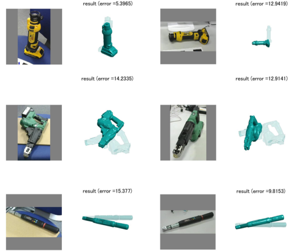
Fig. 6. The results of pose estimation using the test dataset are shown. The Webcam dataset was used for training.
