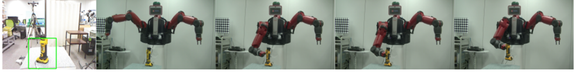
Fig. 9. Baxter robot performing the grasping action.
