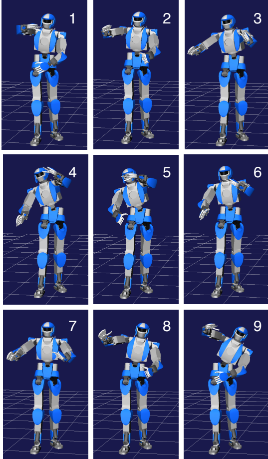
Fig. 9. Scenario 5: Snapshots of the retargeted motion with the humanoid robot HRP-4
