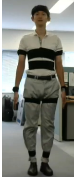
Fig. 6. Initial pose. This step is needed to synchronize the sensors to the software. The position of the IMUs and initial orientation are pre-determined.
