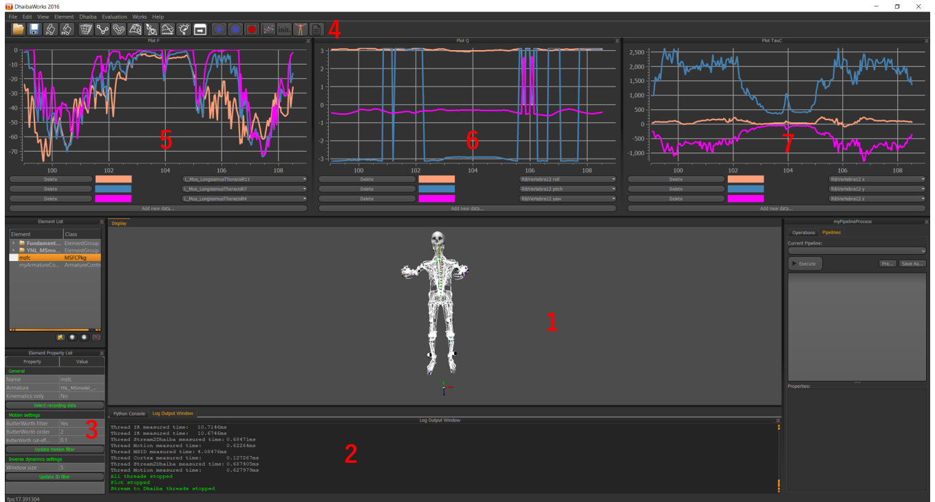
Fig. 8. DhaibaWorks with the integrated plugin. The plugin adds several tools to the main window. It adds 1) visualization of the musculoskeletal model, 2) information into the console on the state of the software, 3) tunable parameters such as filters, 4) toolbar buttons to easily play, record, initialize the software 5-7) plots to visualize on-line state. 5) show 3 back muscles (Longissimus Thoracis 11, 7, 4), 6) is the rib vertebra 12 orientation (roll, pitch, yaw) and 7) show joint reaction forces of the rib vertebra 12 (x, y, z).
