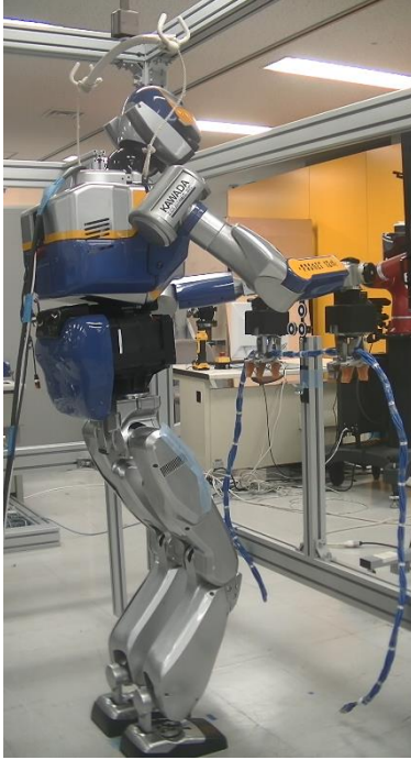
Fig. 2: HRP-2Kai is installing a cable on the first industrial cable clamp.
