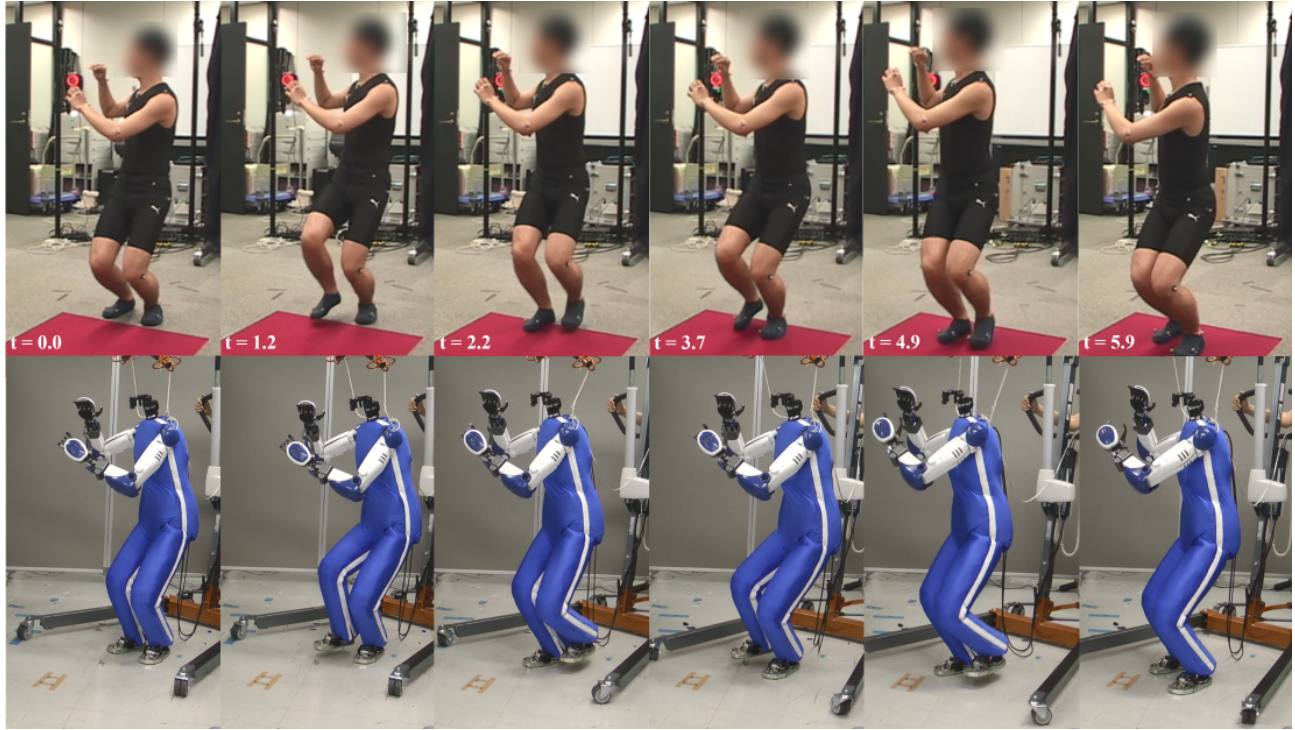
Fig. 6. Original human motion (top) and reproduced motion on HRP-4 (bottom). The motion includes four steps, and the timing of snapshots are the start and end, and each leg swinging.
