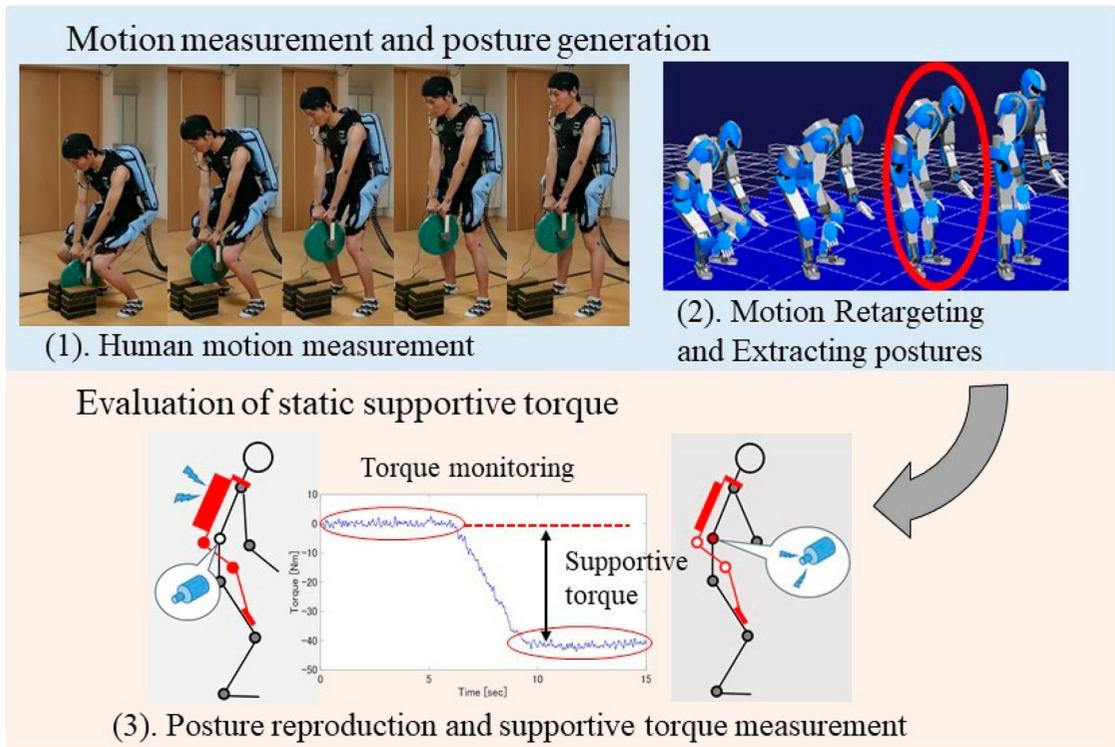
**Figure 1.** Overview of the proposed evaluation framework. (1) Trajectory of human motion when using the assistive device is captured using a motion-capture system. (2) Typical postures when using the device are extracted from the humanoid motion trajectory generated by the motion retargeting method. (3) The supportive torques of device are estimated by comparing robot joint torques with and without device support while the robot reproduces the extracted postures.
