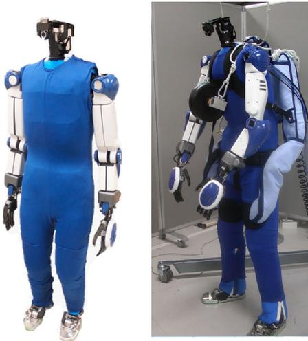
**Figure 7.** Humanoid robot HRP-4 and robot wearing Muscle Suit.
