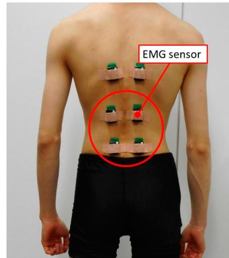
**Figure 5.** Placement of electromyography (EMG) measuring equipment.
