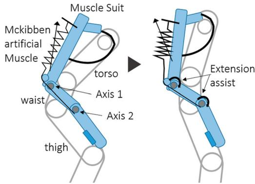
**Figure 3.** The specific structure of muscle suit.
