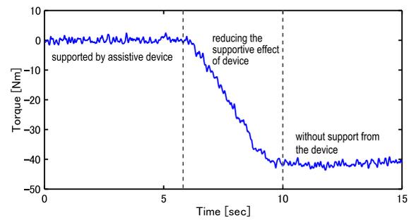
**Figure 10.** Torque measurement result in posture 1 with 10 kg weight.
