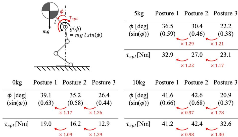
**Figure 11.** Relation between supportive torque  $\tau_{spt}$  and waist joint angle with respect to vertical axis from floor in case of adding no weight (0 kg), 5 kg weight and 10 kg weight. The rates of increase are shown between each value with red colour. They show that the increase in torque corresponds to the increase in angle.
